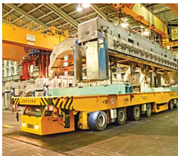
Removal and transfer of superstructure on to the multi-wheeler
