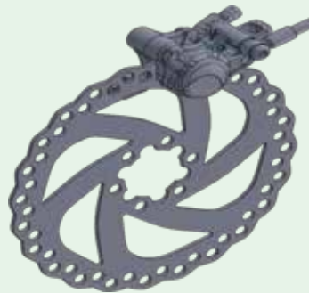
Brake caliper and rotors (disk) interface with the wheel assembly
